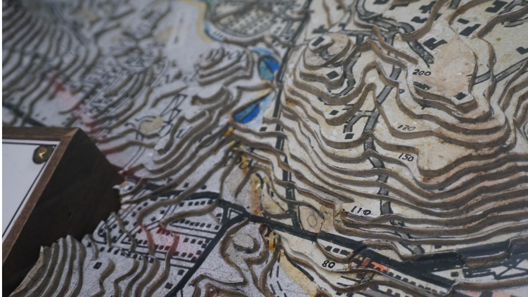
Figure 8. Yellowed, failing adhesive on the relief map.
