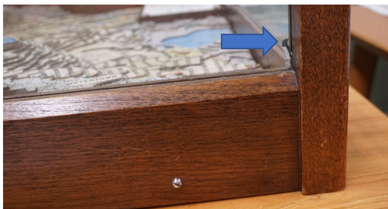
Figure 7. Break in glass siding and light scratching on oak frame.
