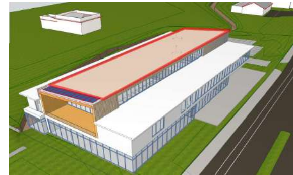
Figure 6: Potential available roof area for PV array
